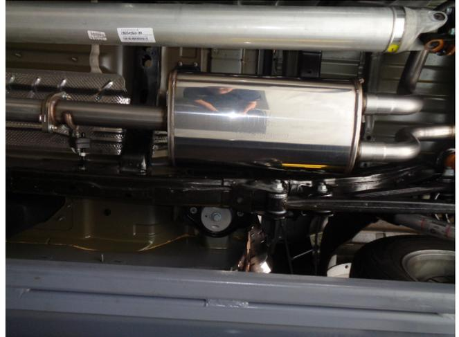
Step 3: Install the new system by attaching the muffler assembly to the resonator pipe assembly with supplied hardware and gasket.
