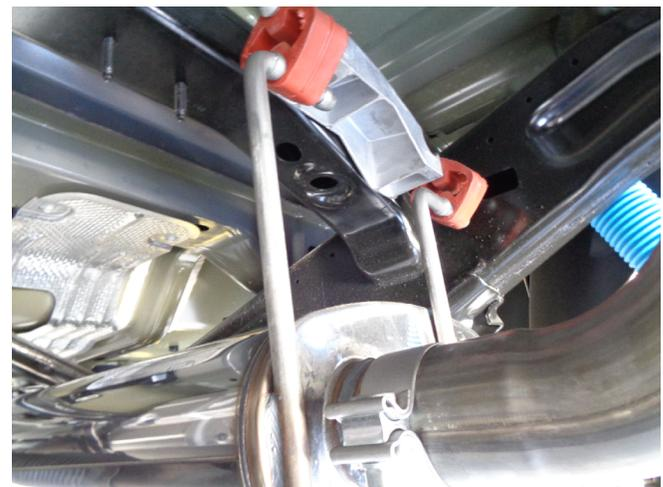
Step 4: Locate the welded hangers to the rubber insulators. Leave all clamps loose for final adjustment of the complete system once installed.
