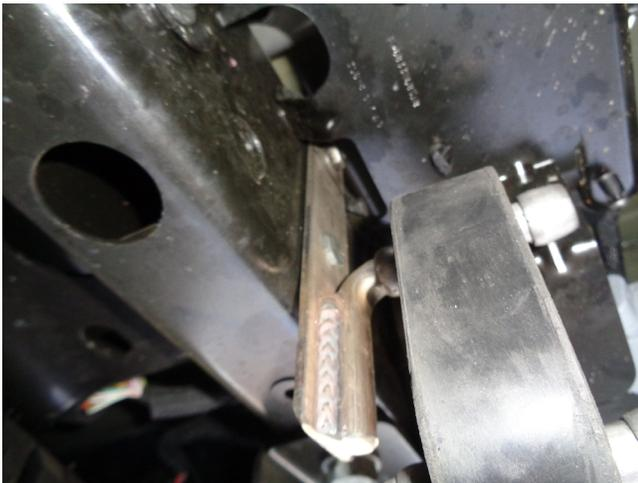
Step 6: On the driver side attach the bracket assembly with the bolts and washers provided.
